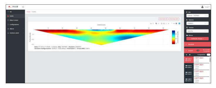
Possibility of **soil water content calculation** based on a relationship derived from resistivity values and water content values of extracted core samples in the monitoring site.
