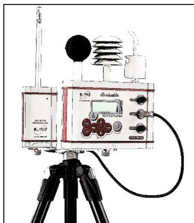
Fig. 7 - Usage of WBGT 1 env. with hot wire anemometer.
