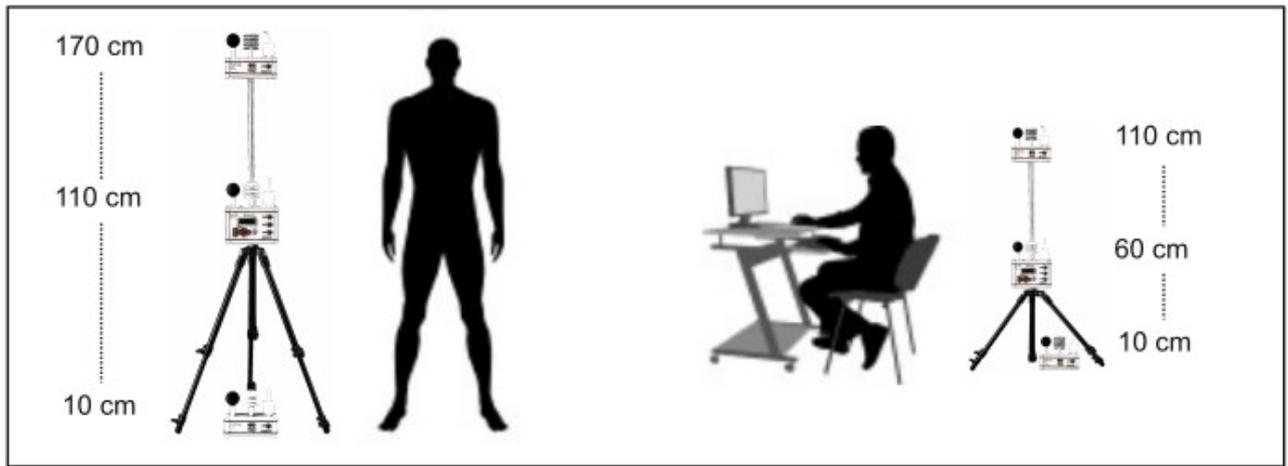
Fig. 3 - Installation of the units in case of WBGT Subject.
