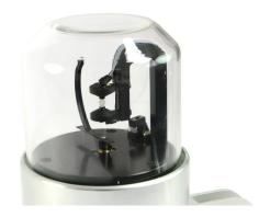
• On each rotation of the band accross the photovoltaic sensitive element, the instrument determines the maximum and minimum values equivalent of the two radiation levels of the beam (global and diffuse irradiances), when the two levels difference (called Direct radiation) is more than 120 W/m², the sensor gives an stutus "on" for the sunshine.
