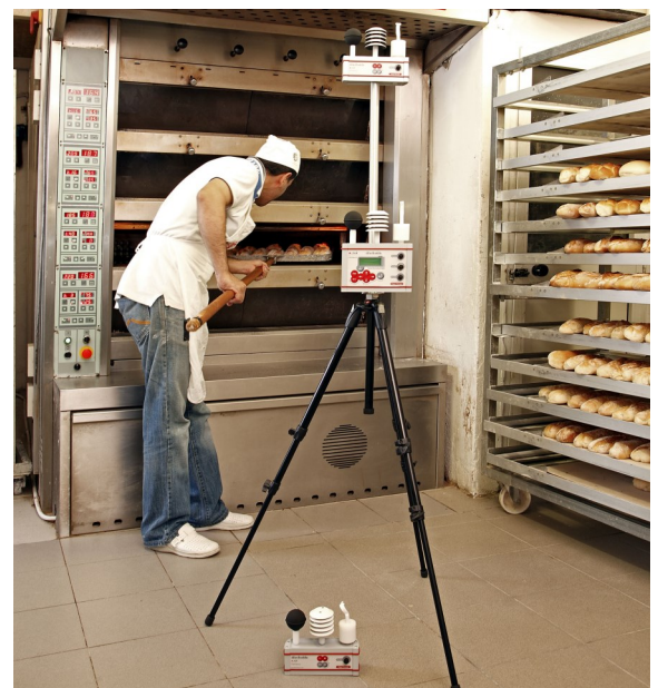
Three levels WBGT on the same vertical
