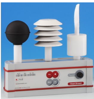
ELR610S: 5 cm diameter black globe sensor satellite modules
